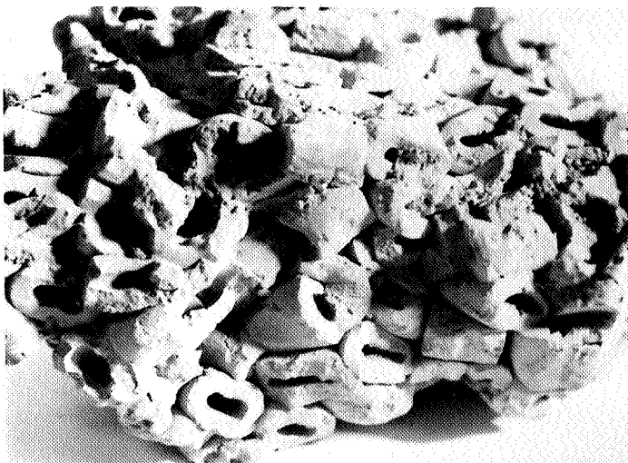
Figure 4. Deformed catalyst taken from the lower one-fourth of the bed.
