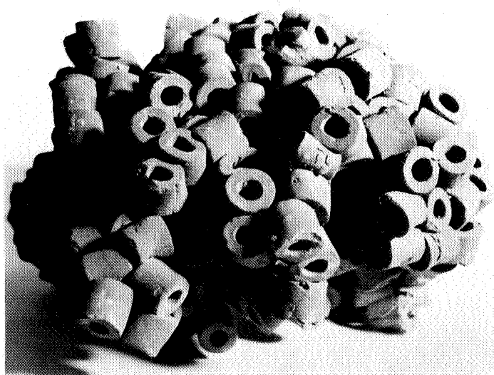
Figure 1. Slightly fused, shrunken catalyst taken from the upper one-third of the bed.
